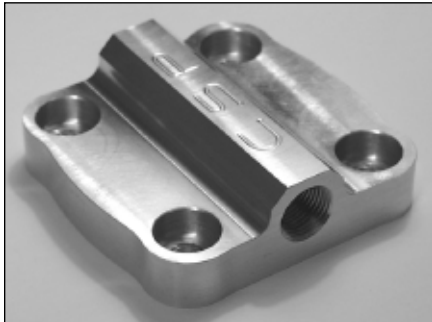
Pump cover modified for outlet, system "2." Return is at boss on third piece, where outlet is on system 1. Below from left: CSP unit, Skirmants' unit with integral pressure relief, welded tach drive cover. Bottom: The original oil system, shown at op temp, and a ssystem 2 with external filter and cooler.
