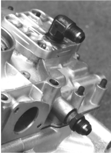
Pump cover modified for outlet, system "2." Return is at boss on third piece, where outlet is on system 1. Below from left: CSP unit, Skirmants' unit with integral pressure relief, welded tach drive cover. Bottom: The original oil system, shown at op temp, and a ssystem 2 with external filter and cooler.
